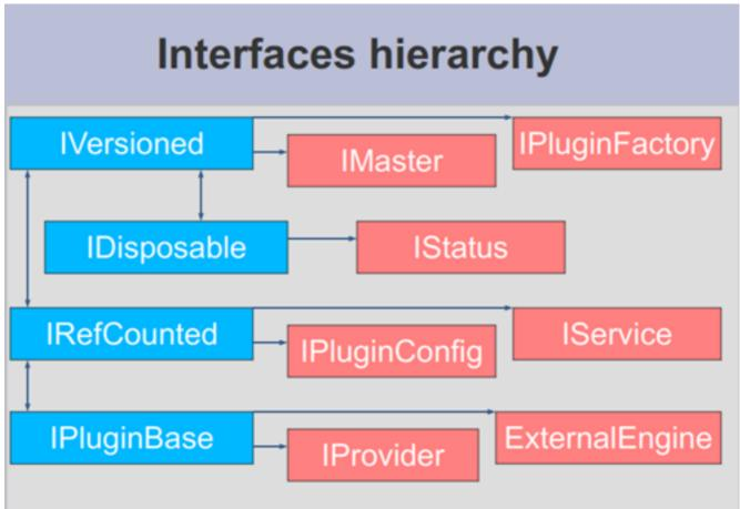
The base of the structure is **IVersioned**. It is the interface that enables a version upgrade. A lot of interfaces not requiring additional lifetime control are based directly on **IVersioned**. **IMaster** is one example already mentioned. Others include a number of callback interfaces whose lifetimes must match the lifetimes of the objects from which they were to be used for callback.
